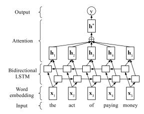
Figure 3.4: The bidirectional LSTM model with a self-attention mechanism.
