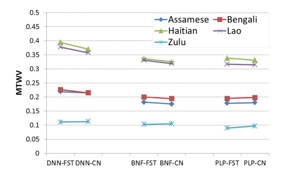
Figure 5.3: System comparison between different ASR systems and search methods.
