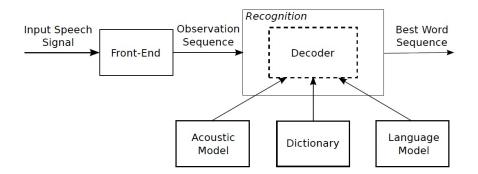
Figure 3.1: General framework for an ASR system (from (Qin, 2013))
