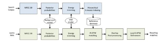
Figure 3.5: An example system framework for a query-by-example STD system (from (Anguera et al., 2013))
