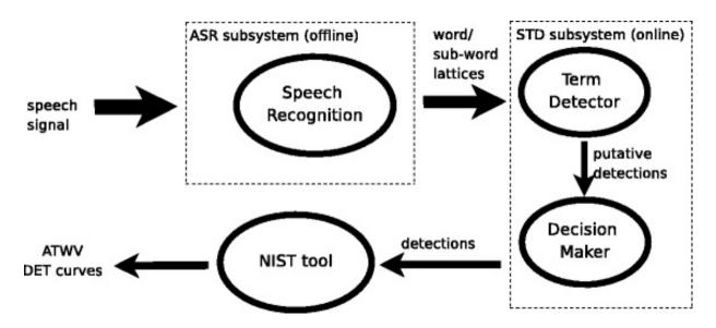
Figure 3.4: Typical STD system architecture and evaluation pipeline (from (Tejedor et al., 2015))
