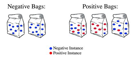
Figure 5.3: Illustration of the label assumptions under the MIL framework. Adapted from **II**.
