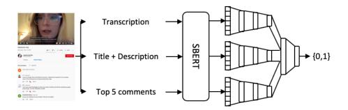
Figure 5.7: Architecture of the fully supervised model that estimates the upper bound of the performance that can be obtained in labeling the WSM Corpus, given the feature choice and model architecture.
