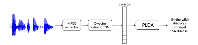
Figure 6.3: Framework, using x-vectors as the front-end and PLDA as the back-end, to detect SA diseases.
