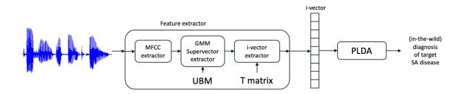
Figure 6.2: Framework, using i-vectors as the front-end and PLDA as the back-end, to detect SA diseases.
