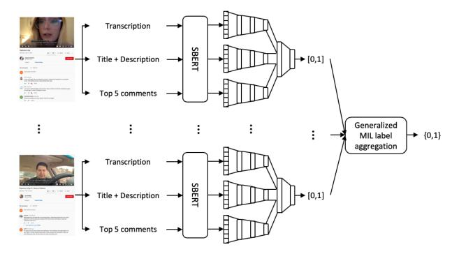
Figure 5.10: Architecture of the proposed deep- $\theta$ -MIL solution to automatically annotate the WSM Corpus. This architecture is based on a 3-stream network, where each stream processed one document.
