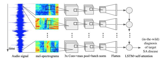
Figure 6.4: Proposed end-to-end model: this model uses mel-spectrograms as inputs to a CNN-LSTM network, where the LSTM layer has a self-attention mechanism.
