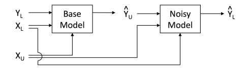
Figure 5.1: Proposed framework, using base and noisy model, to reconstruct labels of the labeled subset of a corpus and estimate labels for the unlabeled subset of a corpus.
