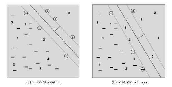
Figure 5.5: mi-SVM (left), and MI-SVM (right) solutions to an arbitrary MIL problem, where negative instances are denoted by "-" and positive instances by a number encoding their bag membership. Adapted from [2].
