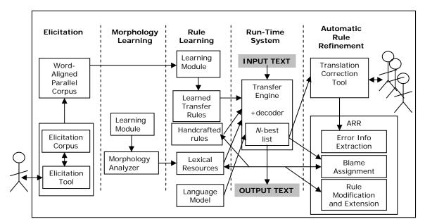
Figure A.1. AVENUE MT System Architecture Diagram.
