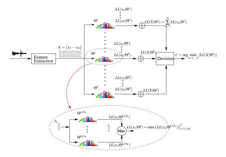
Figure 2.9: Speaker recognition procedure with FSC
