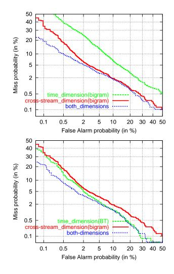
Figure 3.9: Combination of Cross-Stream Dimension and Time Dimension: (upper) LSPMs are bigrams in both dimensions; (lower) LSPMs are bigrams in time dimension and binary trees in cross-stream dimension
