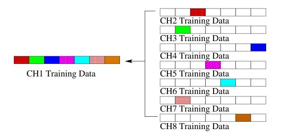
Figure 2.7: Illustration of Data Combination on 3D DMD
