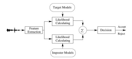
Figure 1.3: Speaker detection system framework
