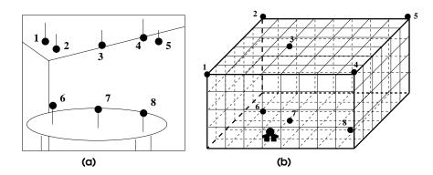
Figure 2.1: Microphone setup in 3D DMD collection
