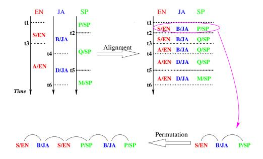
Figure 3.6: Temporal Alignment and Permutation of Multiple Phone Sequences
