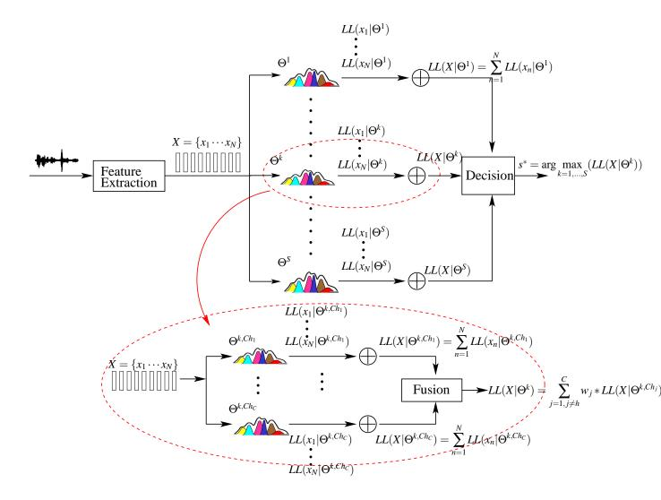
Figure 2.10: Speaker recognition procedure with SSF
