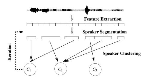
Figure 1.4: Speaker Segmentation and Clustering System Flow
