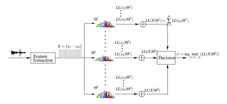
Figure 2.8: Standard speaker recognition procedure
