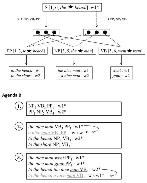
Figure 3.4: Illustration of the second-pass of the Left-to-Right search algorithm. The result of the first pass is the hypergraph rooted at goal item item S. The hypergraph structure and agenda items are explained in the text.
