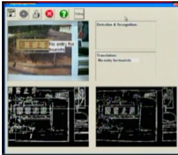
Figure 3.5.1: An early prototype for indoor road sign (printout) recognition. Functions include near real-time road sign detection, text recognition and Chinese-English translation. Bottom windows show intermediate results.
