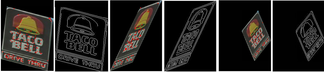
Figure 4.3.1: An example of synthesized views for Taco Bell sign, and the extracted keypoints and edge features for these views.
