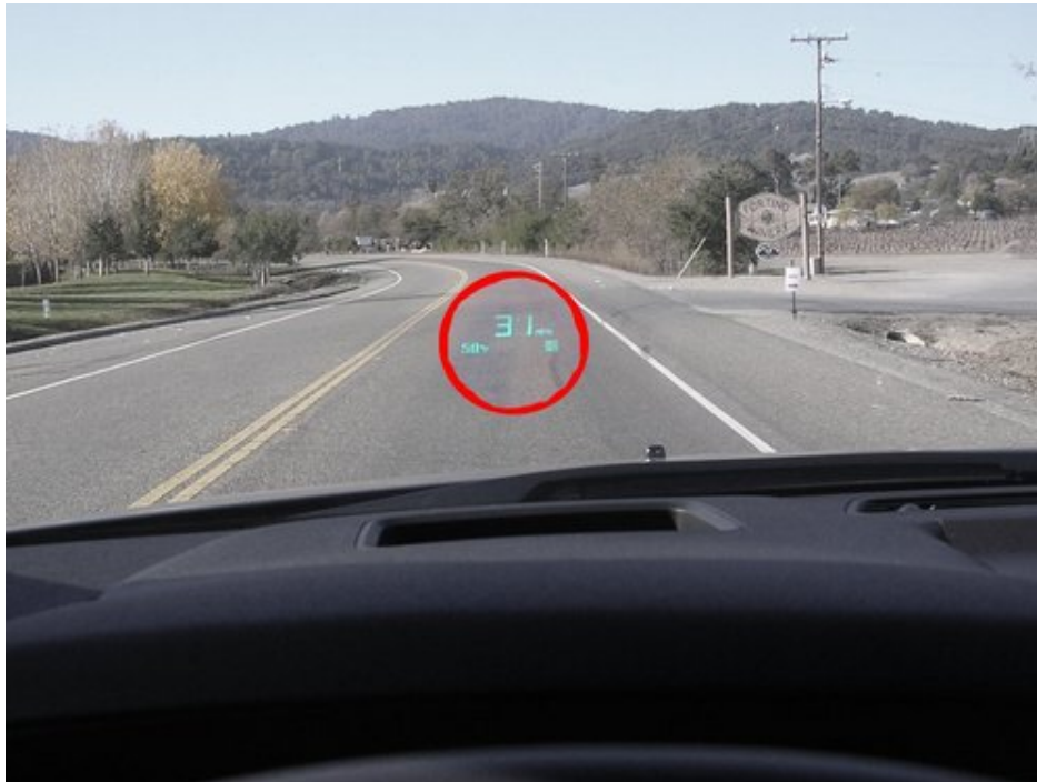
Figure 6.3.1: GMC Acadia Full-Windshield Display showing speed and other information.
