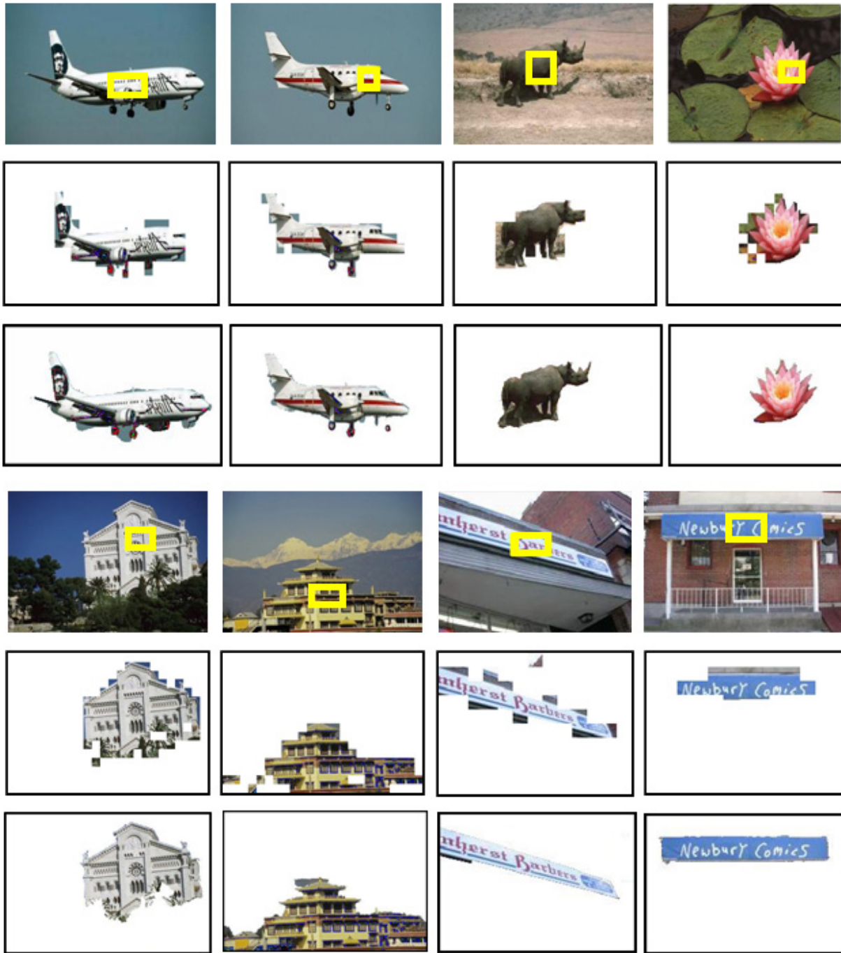
Figure 2.5.4: Comparison between SmartLabel [121] and SmartLabel-2. In two groups of three rows. The 1st row shows input images with ROIs. The 2nd row shows results by SmartLabel. The 3rd row shows results by SmartLabel-2. Two merits of SmartLabel-2 compared to SmartLabel: 1) smooth object boundaries instead of zigzag lines and 2) less misclassified patches.
