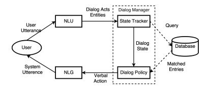
Figure 2.1: Dialog system pipeline for task-oriented dialog systems
