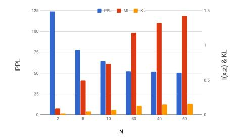
Figure 6.3: Perplexity and  $I(\mathbf{x}, \mathbf{z})$  on PTB by varying batch size *N*. BPR works better for larger *N*.
