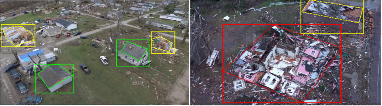
Figure 2.2: Visualization of our ISBDA dataset. The green, yellow and red polygons denote damages in Slight, Severe and Debris levels, respectively. The rectangles composed of solid lines represent damaged building bounding boxes. The polygons with dotted lines represent segmentation masks of damaged parts.
